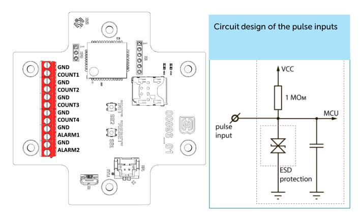
De-bouncing logics with 5 msec time constant is integrated in the pulse counter. The pulse counting is carried out for frequencies up to 200 Hz.
